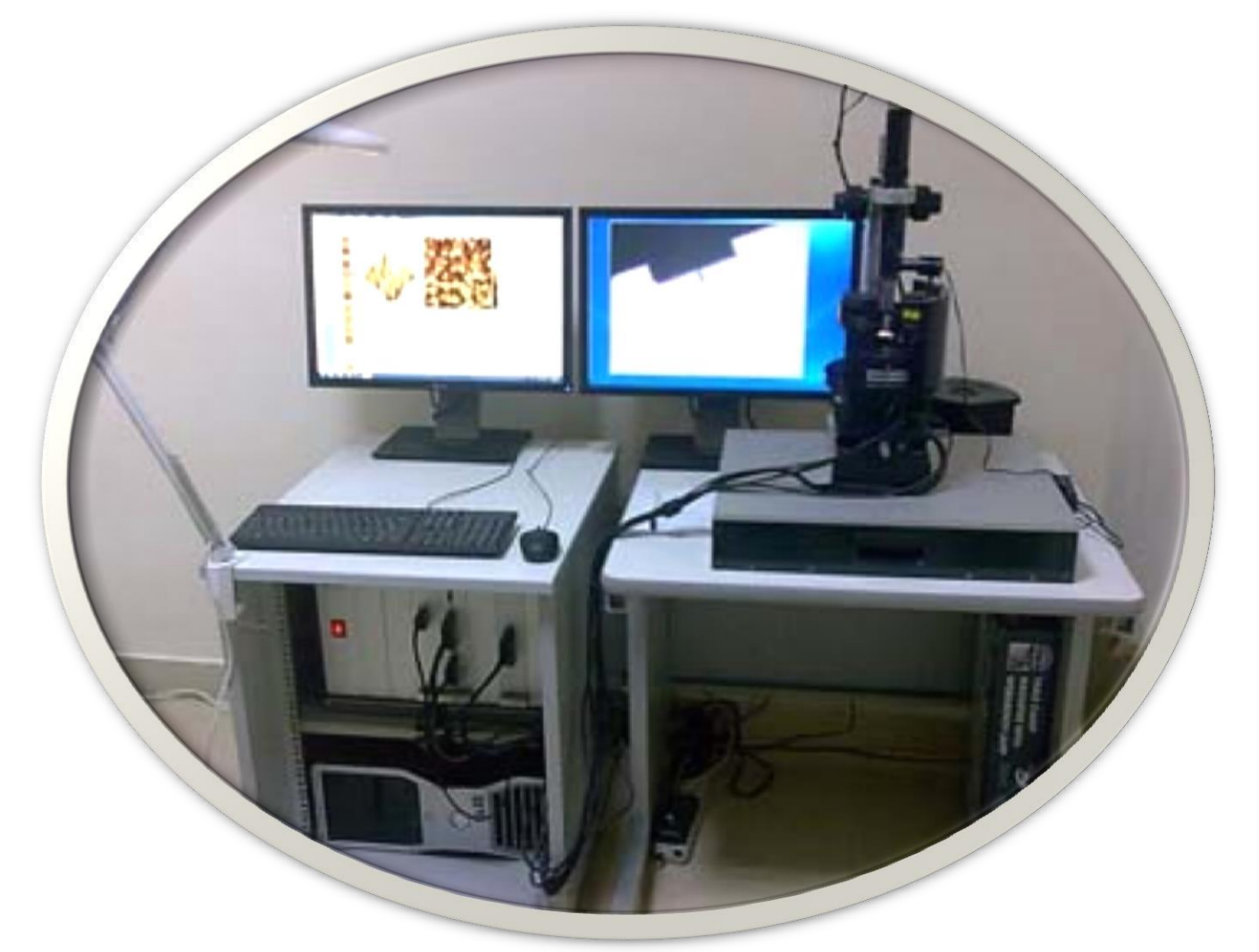
Scanning Probe Microscope (SPM) AIST-NT (Tokyo Instr., Japan)
