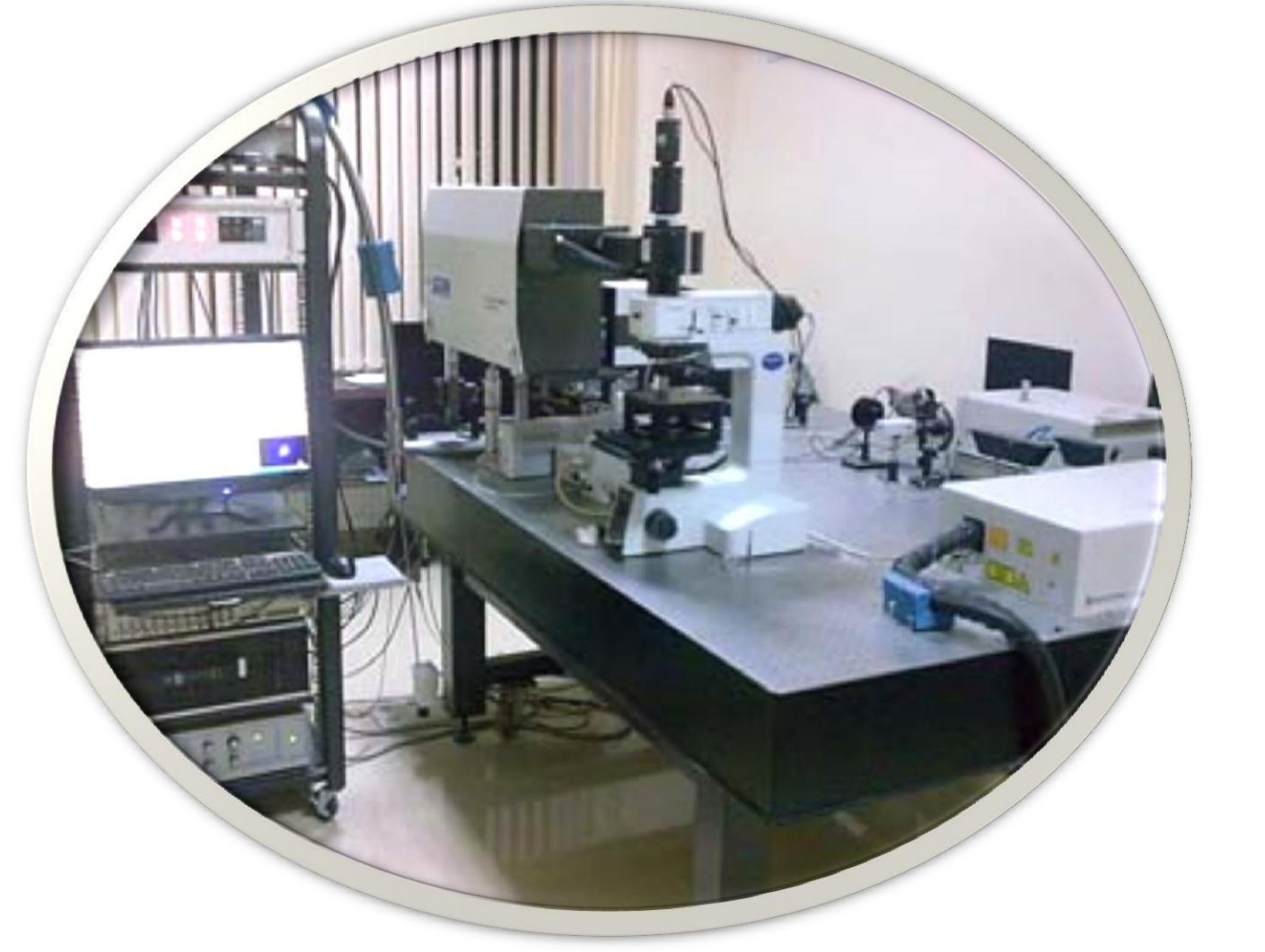
3D Raman Microscopy System, Micro-Nano Scale Micro spectroscopy Nanofinder@30 (Tokyo Instr., Japan)
